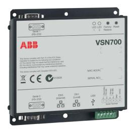
The high-performance VSN700 Data Logger provides simple and quick commissioning with device discovery and automatic IP addressing as well as remote management features.
