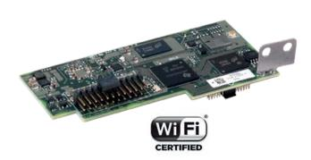
The VSN300 Wifi Logger Card is an advanced expansion board for ABB's UNO and TRIO string inverters\* which provides residential and commercial users with an advanced and cost-effective solution for monitoring and controlling their photovoltaic system.
